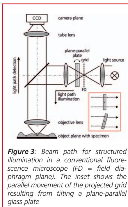
**Figure 3:** Beam path for structured illumination in a conventional fluorescence microscope ( $FD$  = field diaphragm plane). The inset shows the parallel movement of the projected grid resulting from tilting a plane-parallel glass plate
