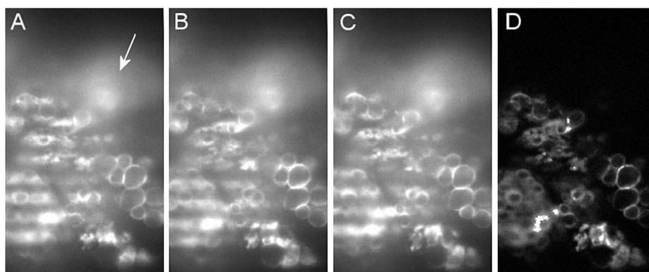
**Figure 4:** For structured illumination, three raw images (at least) are acquired, each with a different grid position (A-C). An image-analysis algorithm calculates an optical section (D) from the raw images online
