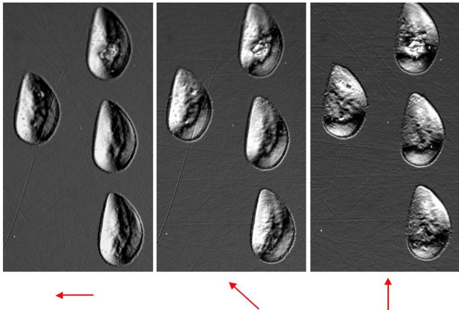
Fig. 12. Excimer laser ablation: signature mark on an optical surface (sample was kindly provided by Mr. A. Hanssen, Aalen; objective, EC Epiplan–Neofluar 20 × /0.50).
