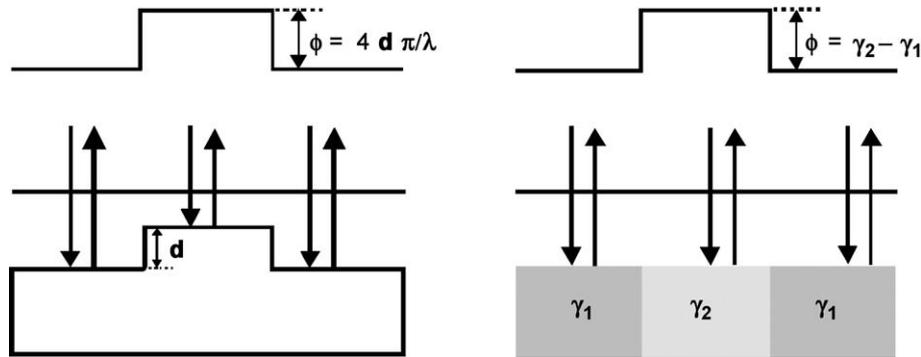
Fig. 1. Geometric (left) and physical (right) incident light phase object: a geometric phase object superimposes the phase difference  $\Phi$  on the reflected light wave front. This phase difference is only dependent on the step height  $d$ . If the phase object demonstrates no differences in height but different materials, the light wave front is deformed by the difference in the material-specific phase shifts  $\gamma_1$  and  $\gamma_2$ .
