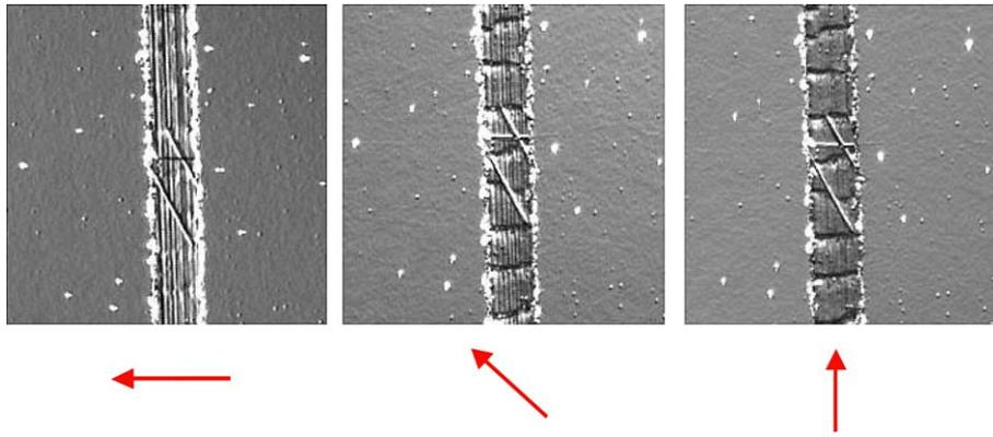
Fig. 11. Synthetically manufactured phase object containing perpendicular phase structures. The arrows indicate the direction of the split (objective, EC Epiplan–Neofluar 20 × /0.50).
