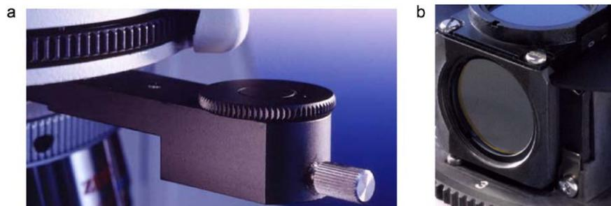
Fig. 9. (a) C–DIC prism slider: the C–DIC prism can be rotated azimuthally using the large knurled ring; the image contrast is varied using the knurled adjusting screw (change to the phase difference  $\psi$ , see text). (b) On both the light entrance and the light exit sides, the C–DIC reflector consists of a polarizer/quarter-wave plate combination arranged crosswise.
