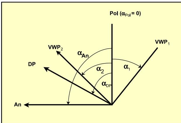
Fig. 8. Diagram illustrating the C–DIC arrangement: unlike in conventional DIC, two further polarization–optical elements, namely the quarter-wave plates VWP1 and VWP2, have been added. Their azimuths  $\alpha_1$  and  $\alpha_2$  are crossed and lie diagonal to the polarizer and analyzer.
