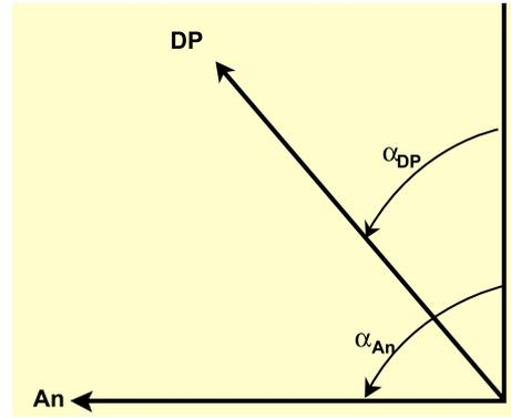
Fig. 6. Conventional arrangement of the DIC prism (DP), in which it must always be arranged diagonally to the polarizer and analyzer so that the interfering waves of ordinary and extraordinary light have equal amplitudes. If this is not the case, the interference contrast is reduced or
