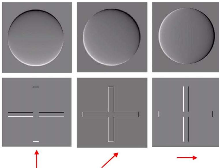
Fig. 5. Top row: circular phase objects can be depicted in high contrast whatever the direction of the split (arrows) of the DIC prism. Bottom row: straight structures show a significant azimuth effect that leads to misinterpretations.
