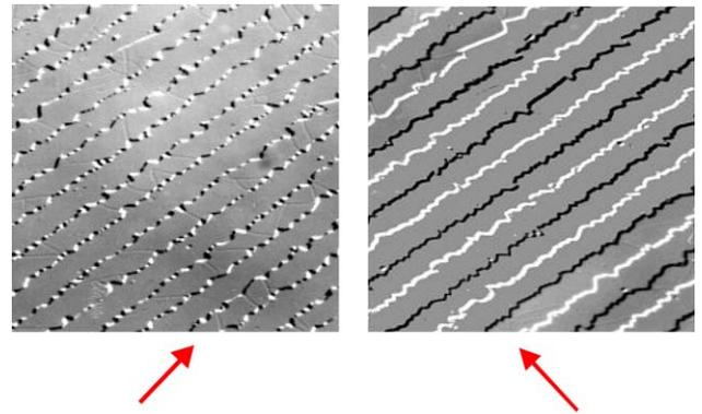
Fig. 10. Images of the same phase object in which the directions of the split are perpendicular to each other. The difference in information is obvious (objective, EC Epiplan–Neofluar  $10 \times /0.25$ ).
